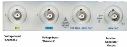
If the cables are not attached, slide the 'notches' in the cable over the 'lugs' seen in the photo and twist about one fourth of a turn clockwise to lock.
