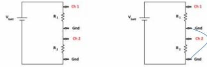
The two ground connections SHORT R2 – you measure  $V_{batt}$  on CH 1 and 0 V on Ch 2.
